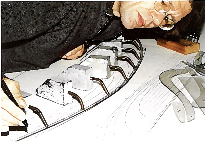
Figure 1. Originally splines were long strips made of very flexible strong material, used as an engineer's tool at the drawing-table. Nowadays the computer has almost completely taken over this design function.
